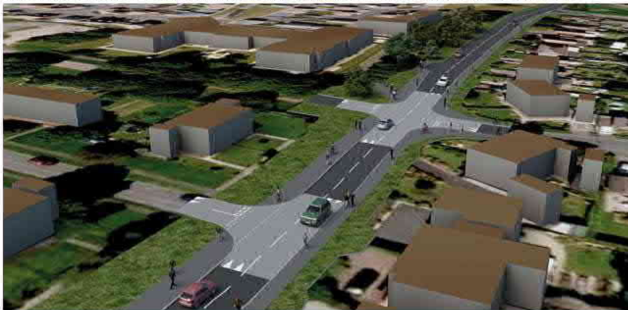
119 Visualisation of possible shared use footway/cycleway either side of Hoarwithy Road at the Aconbury Avenue / Saxon Hall entrance crossroads, looking north towards existing cycleway at Poppy Walk
